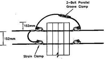
DETAIL OF ATTACHMENT OF OHGW FROM H-FRAME TO TYPE "E" TO H-FRAME
