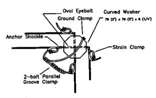
DETAIL OF ATTACHMENT OF OHOW FROM H-FRAME TO TYPE "D" TO H-FRAME
