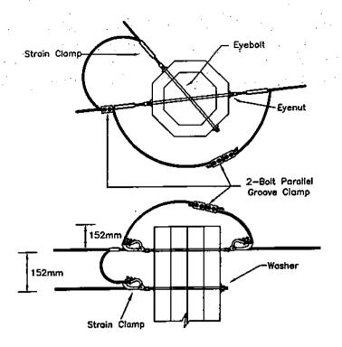
DETAIL OF ATTACHMENT OF OHGW FROM H-FRAME TO TYPE "E" STRUCTURE AND VICE VERSA
