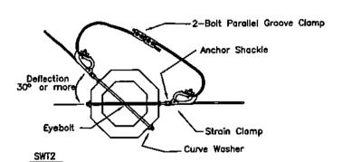
DETAIL OF ATTACHMENT GROUND WIRE ON TENSION STRUCTURE
