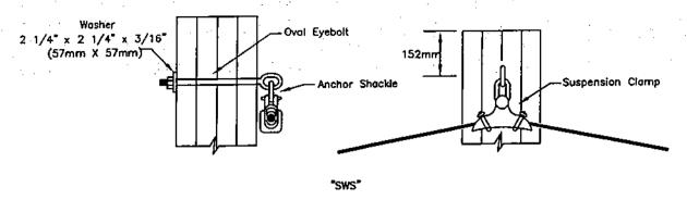
DETAIL OF ATTACHMENT OF OVERHEAD GROUND WIRE ON SUSPENSION STRUCTURE
